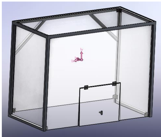
Figure 6. Hood CAD used to Estimate System Weight
